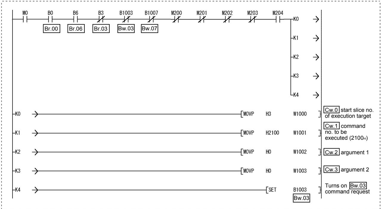
\* The program area enclosed by the dotted line is not required when GX Configurator-ST is used to set the command parameters.
