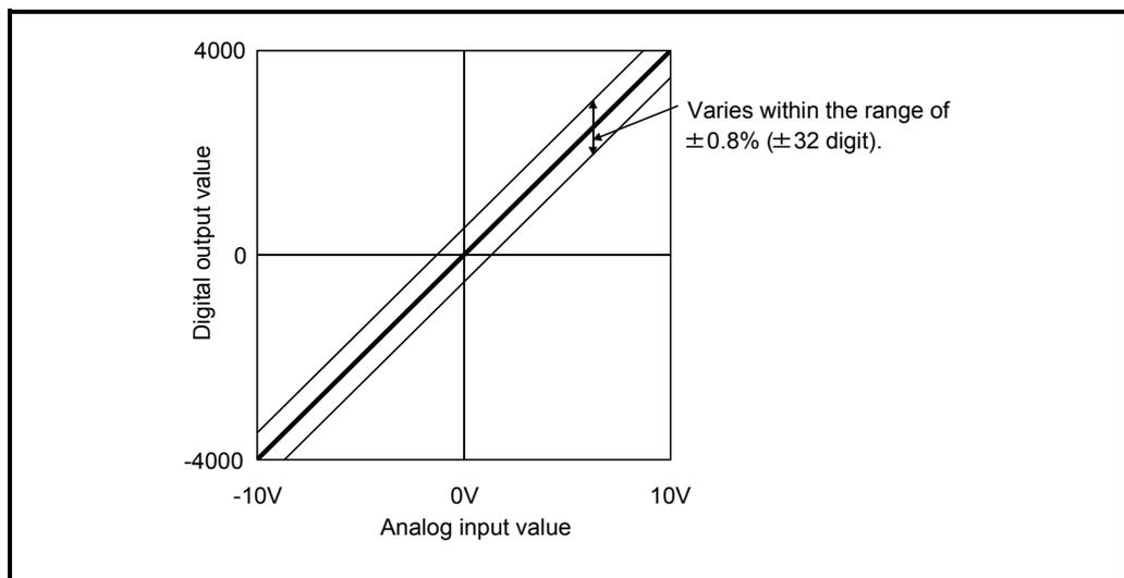
Fig. 3.3 Accuracy of ST1AD2-V
