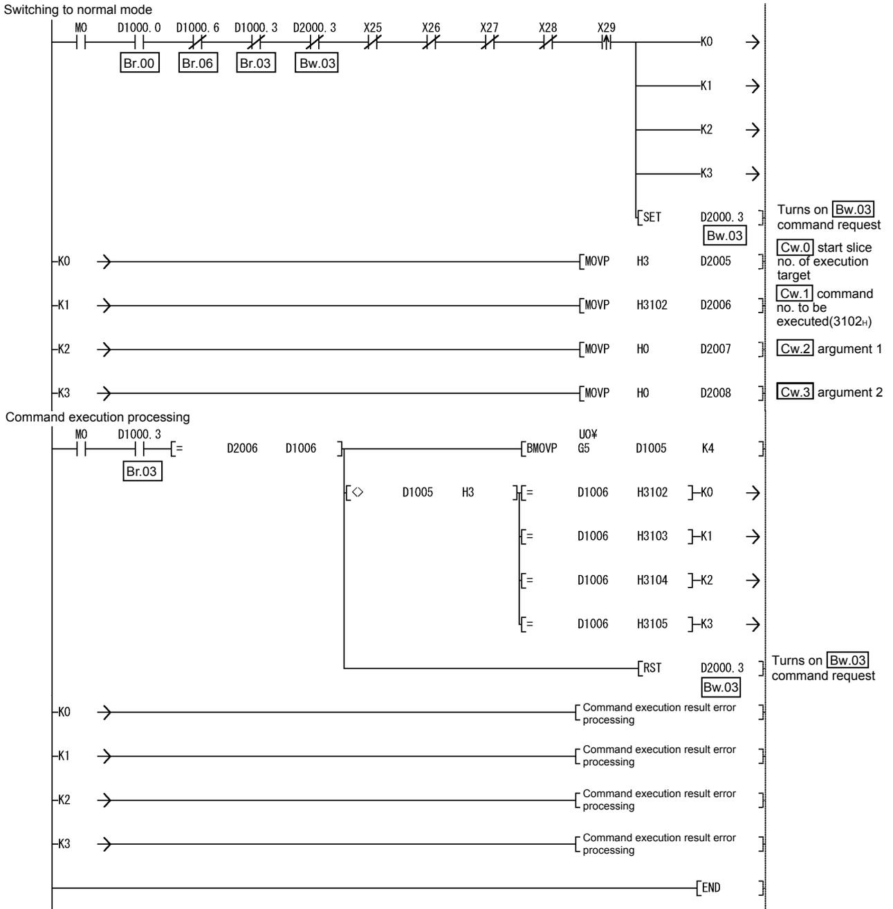
(b) When AJ71PB92D/A1SJ71PB92D is used as master station
