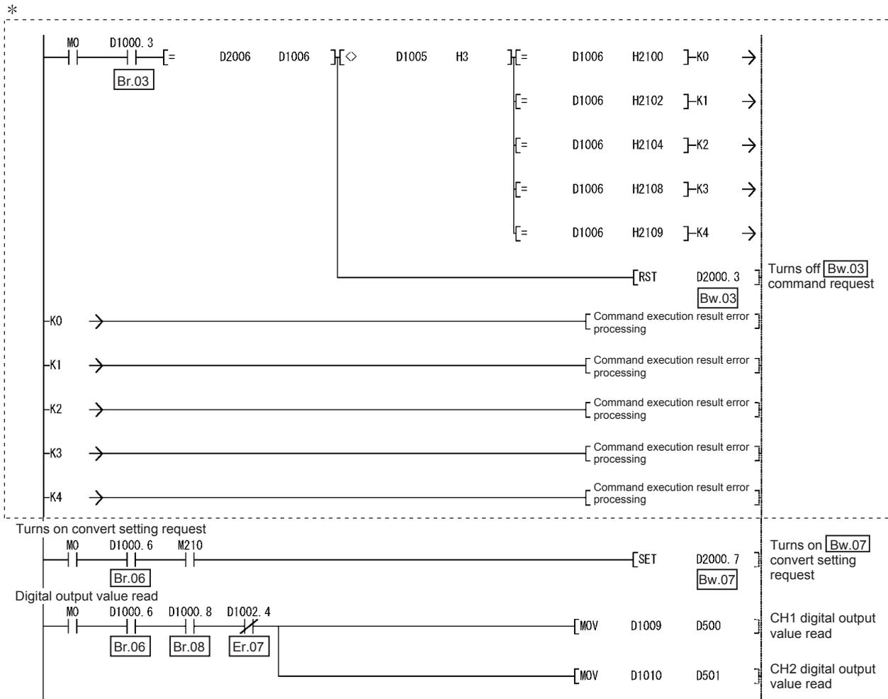
\* The program area enclosed by the dotted line is not required when GX Configurator-ST is used to set the command parameters.
