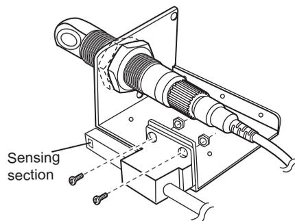
Do not allow anything to touch the metal case of the Sensor Head. Failure to do so might prevent accurate measurement by the sensor.
