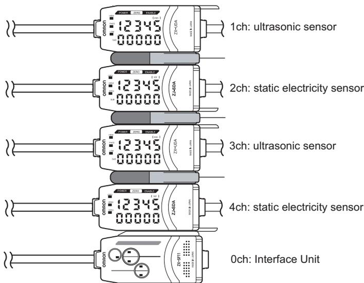
\*(When [Reference destination setting] is set to [Next CH]), the static electricity sensor on 2ch and 4ch can perform correction using the data of the ultrasonic sensors on 1ch and 3ch, respectively.
