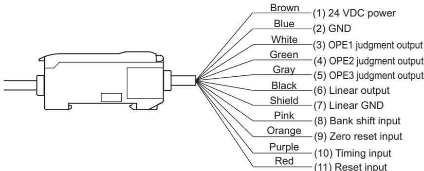
(1) 24 VDC ( $\pm 10\%$ ) power supply is connected to the power supply terminal.
