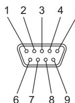
Connect the ZJ-SF11 and the personal computer using a D-sub 9-pin (female-female) cross cable.
