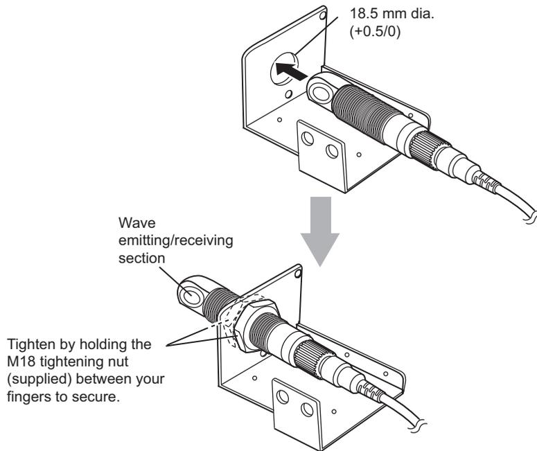
The nut must be tightened with a torque of 45 Nm or less.
