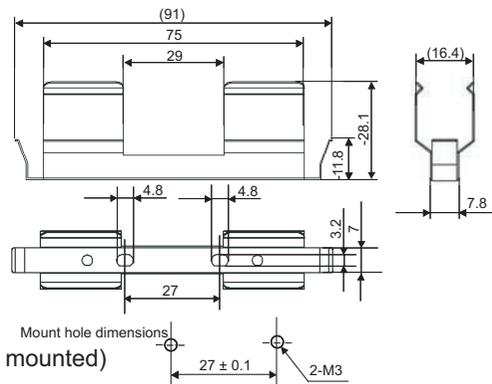
· Preamplifier (when Preamplifier mounting bracket is mounted)
