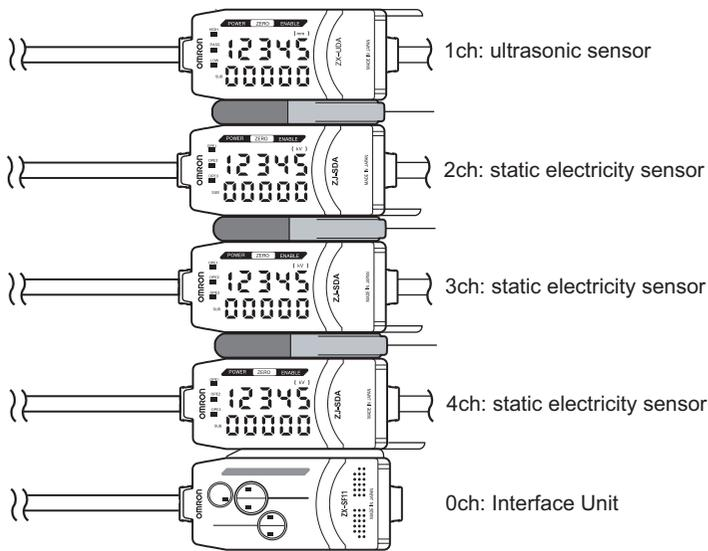
(When [Reference destination setting] is set to [CH1]), the static electricity sensor on 2ch to 4ch can perform correction using the data of the ultrasonic sensor on 1ch.
