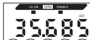
To cancel zero reset from an external device, input the zero reset signal for at least one second.
