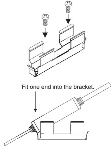
3. Fit the other end of the Preamplifier into the bracket.
