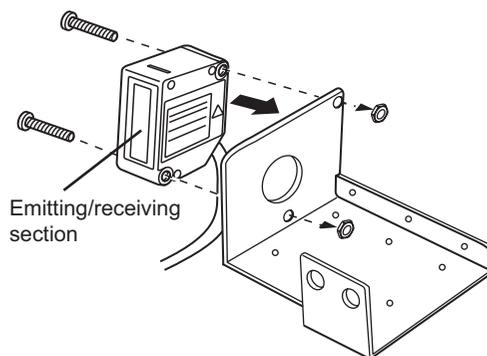
The screws must be tightened with a torque of 0.3 Nm or less.
