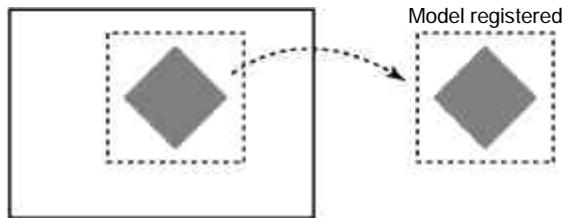
**2** The part of the input image that most corresponds to the model is found. The extent of conformity with the model is expressed as a correlation value. A correlation value between 0 and 100 is displayed. The higher the correlation value, the more similar the input image is to the model. By setting a threshold for this correlation value, OK (acceptable) and NG (unacceptable) products can be distinguished.
