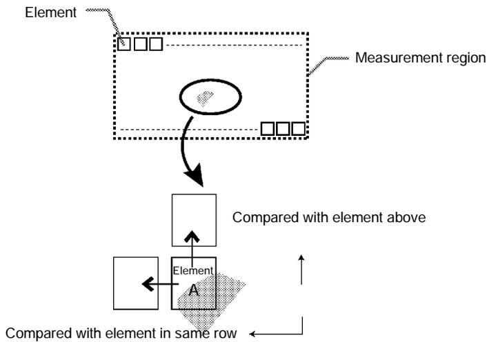
The defect is calculated for all of the elements. If the largest defect is larger than the evaluation criteria, the measurement region is judged to contain a defect. When deciding the evaluation criteria, perform measurements of several samples and base the evaluation criteria on the defects for those samples.
