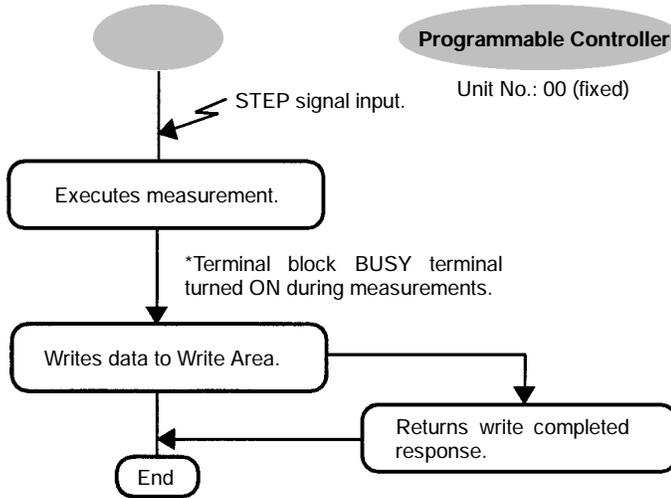
\*A timeout error will occur if there is no response within 5 s. An error message will appear on the screen and the error terminal will turn ON.
