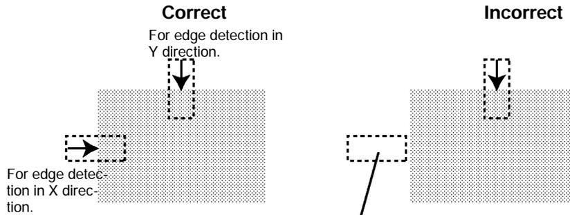
If the edge is not in the measurement region, edge detection will not be possible. Make a region of a size and position that allows for movement of the range of the measurement object.
