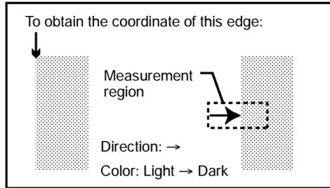
This method can also be used for position displacement compensation.
