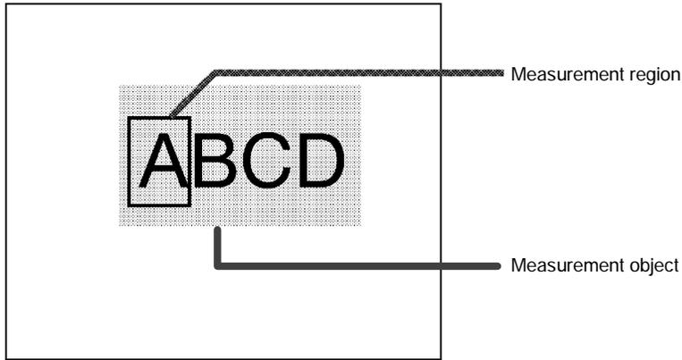
**Measurement Object Displaced**
