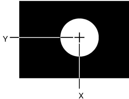
The coordinates for the center of gravity are obtained. These coordinates can be used for position displacement compensation.
