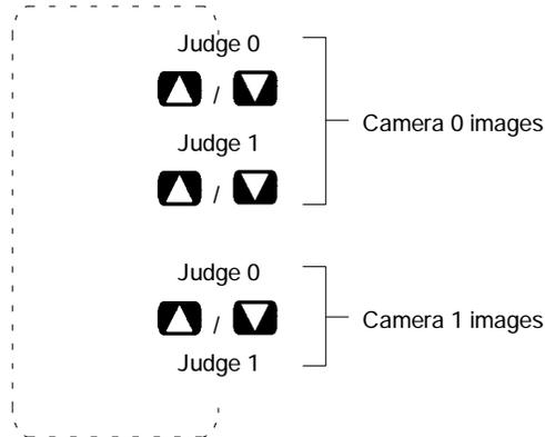
**I/O Monitor** The contents of input made from external devices to the F150 and the contents of output made from the F150 to external devices can be displayed. (The contents of output are only possible in Run mode.)
