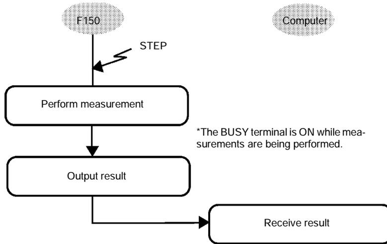
**Note** When RC/CS or Xon/off flow control is selected, if a response is not received from the computer within a set time, the F150 will conclude that there is a disconnection or that the computer is not operating normally, and will generate a timeout error. An error message will be displayed and the error terminal will turn ON.
