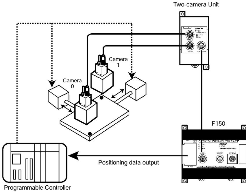
Measurement processing can be performed on images obtained by joining Camera 0 images and Camera 1 images. This means that the image required can be obtained in the time it usually takes to obtain one normal image. (In Horizontal Composition mode 1, however, an extra 8.3 ms is required.)
