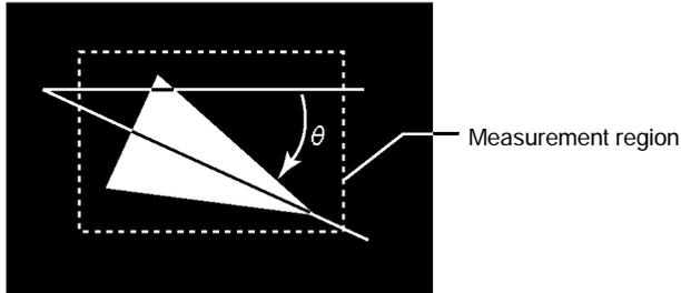
The coordinates for the center of gravity and the axis angle are obtained. This data can be used for position displacement compensation.
