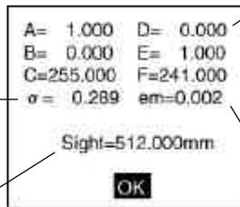
A to F represent the calibration conversion values. The camera coordinates are converted to physical units based on these calibration conversion values. The formulae for conversion to physical units are as follows:
