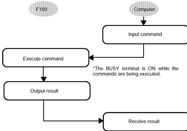
**Note** When RC/CS or Xon/off flow control is selected, if a response is not received from the computer within a set time, the F150 will conclude that there is a disconnection or that the computer is not operating normally, and will generate a timeout error. An error message will be displayed and the error terminal will turn ON.
