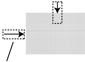
Unless a difference in density that is greater than the set level is detected, position displacement compensation will not be performed. The judgement will be NG.
