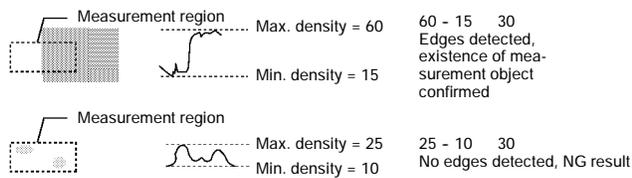
Set the level of density change for identification as an edge. (0 to 100)
