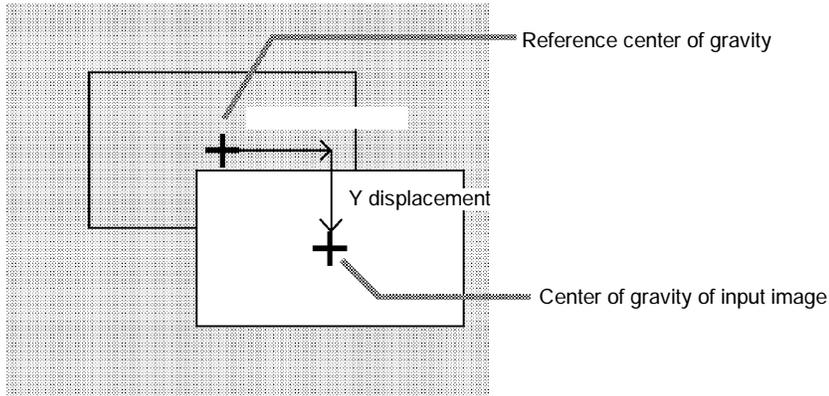
**Binary Center of Gravity and Axis Angle**
