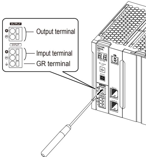
2. With the tip of the flat blade screwdriver in the hole, insert a cable into a round hole at the left of the terminal block.
