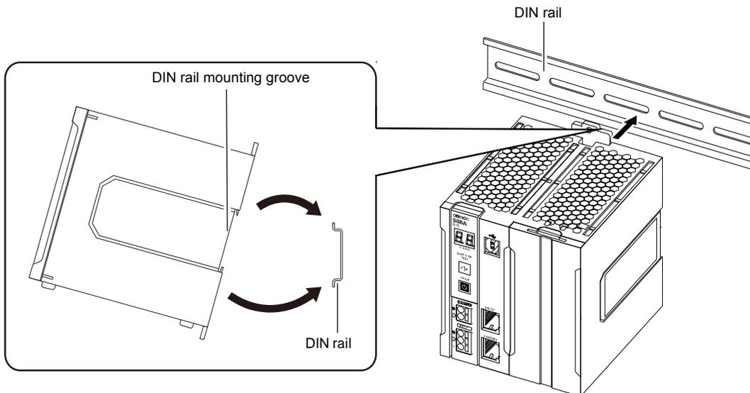
**3.** Close the “DIN rail mounting hooks” in the back of the UPS.
