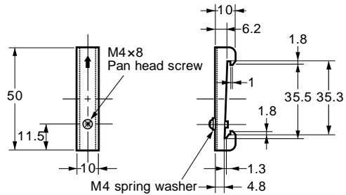
Note 1: If the DIN rail is subjected to vibration or shocks, scrap metal can be produced because of aluminum abrasion. In such a case, use a steel DIN rail instead.
