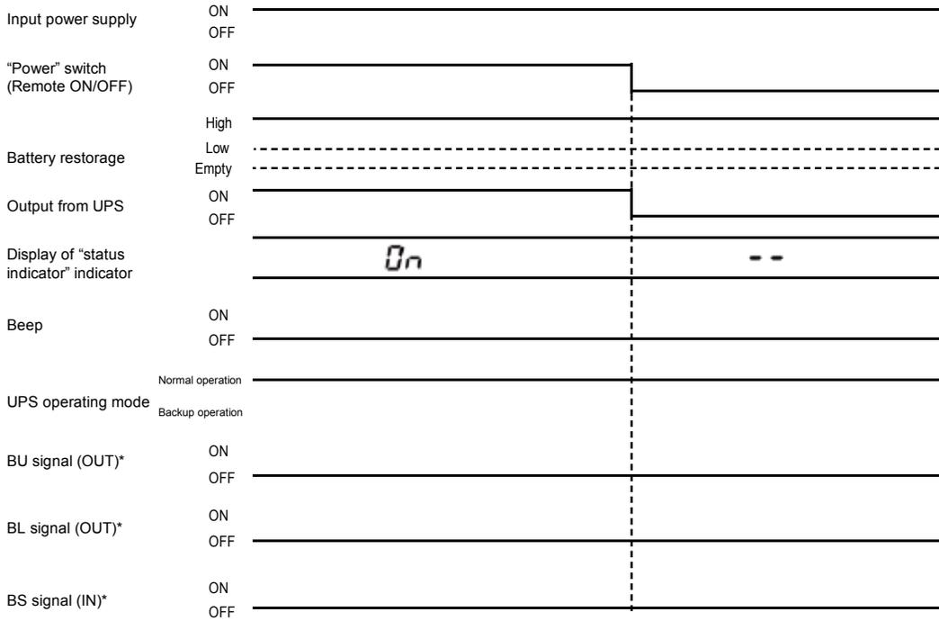
When the "Power" switch is turned OFF during backup operation
