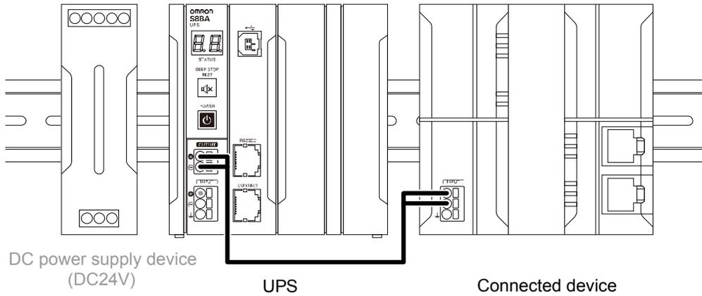
2. When using the UPS monitoring software or the I/O signal, connect the unit to the target device with a connection cable. For details about the connection procedure, see “5 Maintenance and inspection”, and “6 To perform shutdown processing of the devices when a power failure occurs”.
