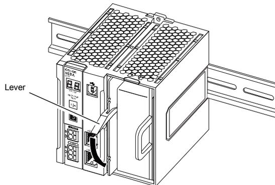
**9.** Hook the lower clamp of the battery cover onto the main unit.
