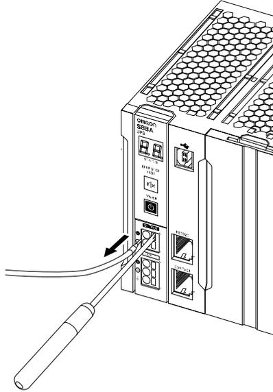
2. Pull out the flat blade screwdriver.
