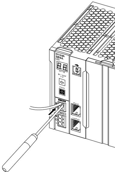
3. Pull out the flat blade screwdriver. Then, the cable is locked.
