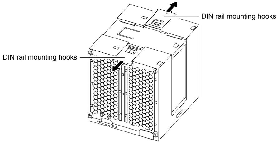
2. Hook the “DIN rail mounting groove” in the back of the UPS onto the DIN rail. Put a hook on the groove on one end ( ), and put the other hook on the groove on the other end ( ).
