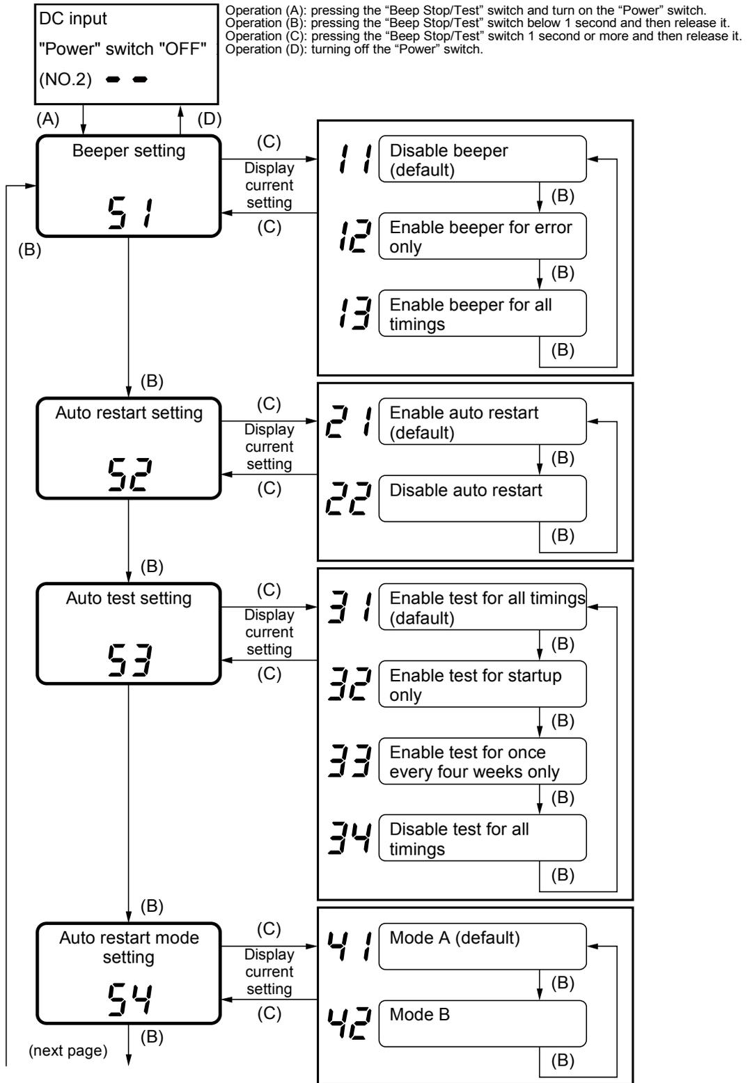
Operation (A): pressing the "Beep Stop/Test" switch and turn on the "Power" switch.
